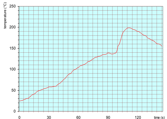
T° measured on the topside of the PCB on a lead-free soldering machine.
